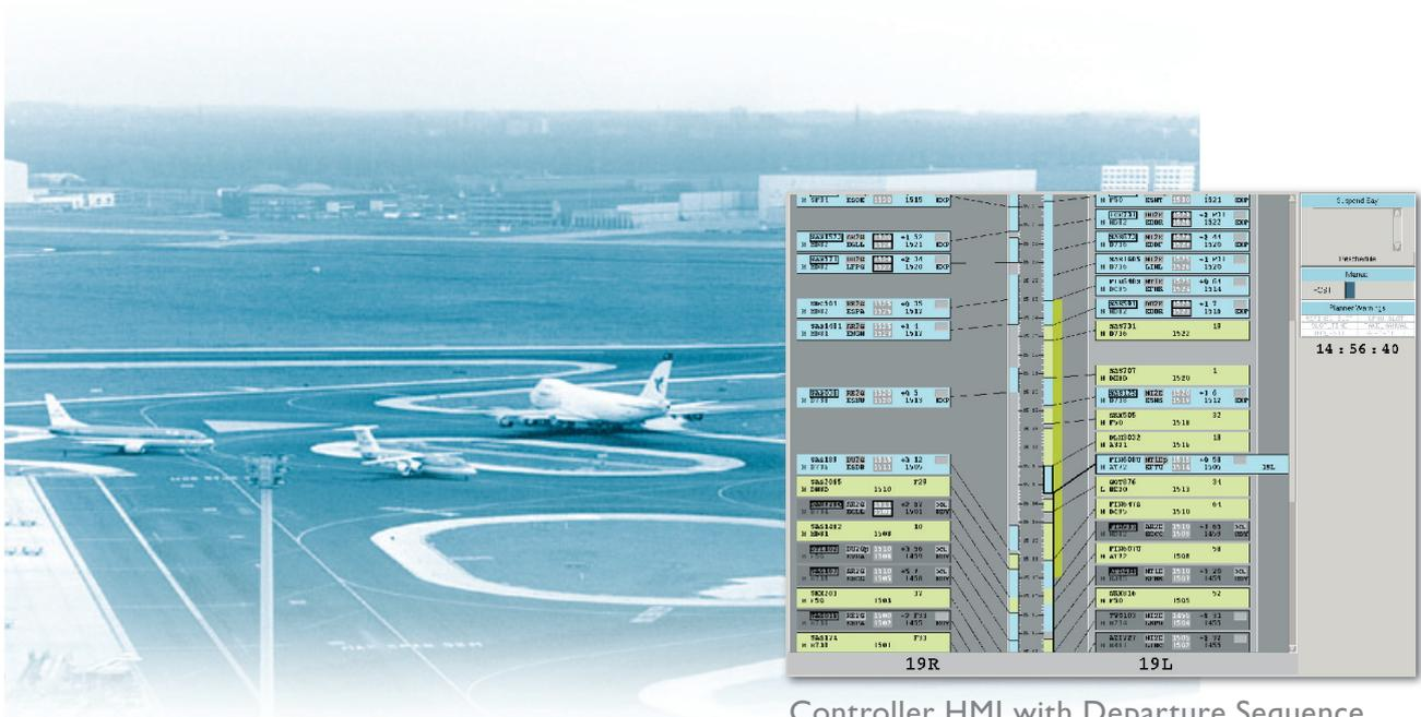
Controller HMI with Departure Sequence (blue labels) in mixed mode operations
